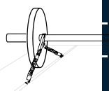
• STEP 3 - Attach Cam Buckle to bar on each side.
